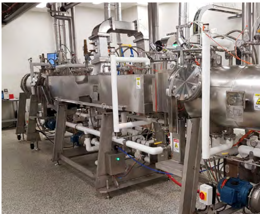
MATS pilot plant pre-heating, microwave and cooling sections. Defence Science and Technology. Scottsdale, Tasmania.
