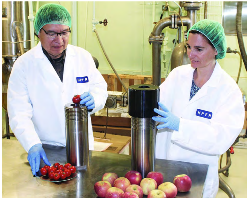
Roberto Avena-Bustillos (left) and Cristina Bilbao-Sainz demonstrate the use of isochoric freezing chambers. Photo U.S. Department of Agriculture.
