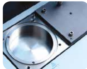
The two separate titanium chambers offer the ability to run the same test in duplicate, or two different tests simultaneously.
